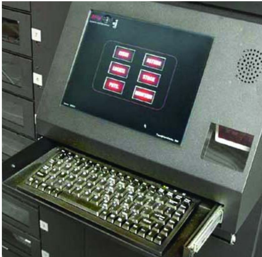
Employees follow RoboCrib's menu prompts to obtain a desired tool. The accountability system has 150 standard reports available that, among other things, can track tool consumption by employee, department and job number.
